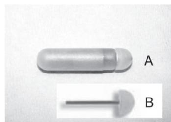
Figure 1. (A) Fully assembled ALZET<sup>®</sup> osmotic pump; (B) flow modulator.
