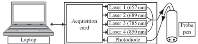
Figure 1. Schematic diagram of the four wavelength optical probe.
